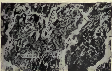
FIG. 13.—(Stoughton.) Meshes of pearlite in a network of cementite from hyper-eutectoid steel. Magnified 250 diameters.
